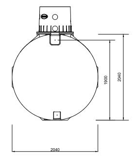
Standard detail using Tank Dome Maxi. For different accessories, please refer to detail below or contact Graf UK for support. NOTE:-
