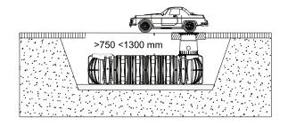
Cover heights with HGV-bearing telescopic dome shaft
