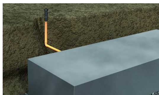
Figure 15: Fitting the vent
