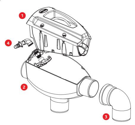
5. ASSEMBLY OF THE GRAF MINIMAX-PRO FILTER INTERNAL
