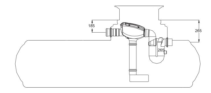
5. ASSEMBLY OF THE GRAF MINIMAX-PRO FILTER INTERNAL
