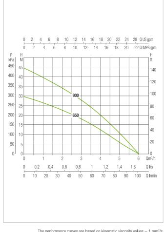
The performance curves are based on kinematic viscosity values = 1 mm<sup>2</sup>/s and density equivalent to 1000 kg/m<sup>3</sup>. Curve tolerance according to ISO 9906.
