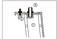
The upper half shell 4 is now positioned onto the lower half shell 1 and the quick connectors 5 are installed. To do this, each 2nd quick connector is pre-adjusted in the 1st step and is secured with a hammer and a wooden support. The quick connectors engage in their end position. The remaining quick connectors are then installed.
