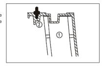
Then insert the centring pins ③ into the intended mountings around the circumference.
