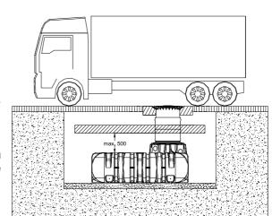
Coverage heights on installation in groundwater – the hatched area specifies the permissible immersion depth for the tank.
